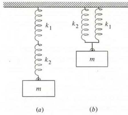
The spring with spring constant  $k_1$  is attached to the ceiling and one end of the spring with spring constant  $k_2$ , and the other end of the second spring is attached to the block (the springs are attached in *series*).
