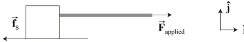
**Figure 7.15:** Forces acting on block and rope
