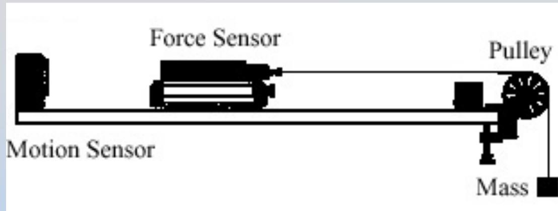
Consider a track with a pulley located at one end. The force sensor and cart have total mass  $m_1$ . They are connected by an inextensible rope of length  $l$  (passing over the pulley) to a block of mass  $m_2$ . You may ignore the small mass of the rope and pulley. You may also assume that all friction effects are negligible. What is the tension in the string both before the cart is released and while the cart is in motion?
