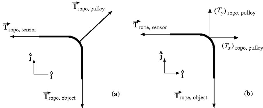
**Figure 8.8.2 (a)** Forces acting on rope with negligible mass
