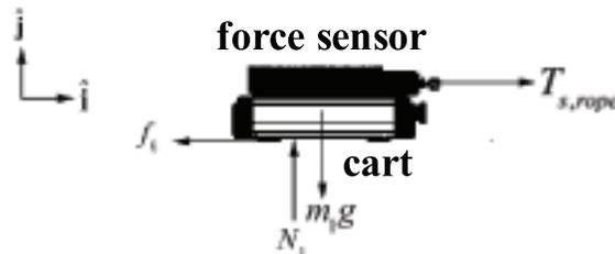
**Figure 8.7** Force diagram on sensor/cart with a vector decomposition of the contact force into horizontal and vertical components
