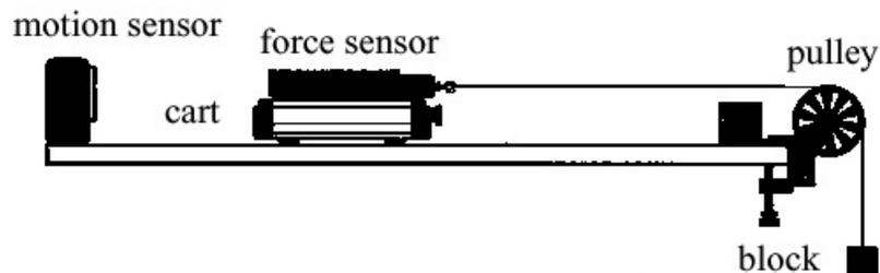
**Figure 8.6** A falling block will accelerate a cart on a track via the pulling force of the string. The force sensor measures the tension in the string.
