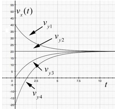
**Figure 8.19** Falling objects with friction
