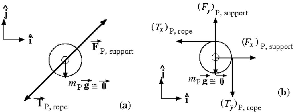
**Figure 8.8.1** (a) Force diagram on pulley (b) Vector decomposition of forces on pulley
