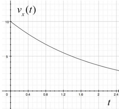
**Example:** An object moving the x-axis with an initial x-component of the velocity  $v_x(t = 0) = v_{x0}$  experiences a retarding frictional force whose magnitude is proportional to the square of the speed (a case known as *Newtonian Damping*),
