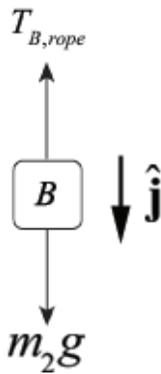
**Figure 8.8** Forces acting on the block
