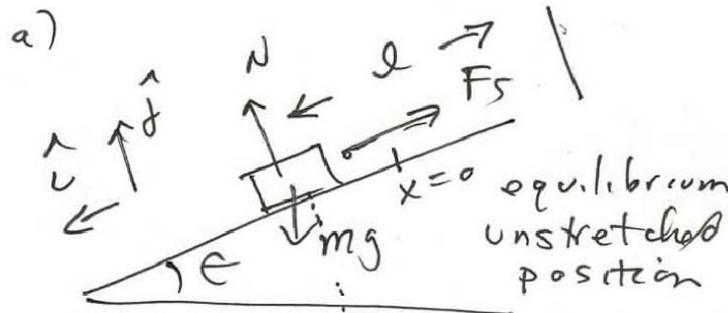
The  $x$ -components of the forces are  $mg \sin\theta$  and the spring force  $-k(l-l_0)$ , with the minus sign indicating that at equilibrium, the spring force is directed up the ramp to hold the cart in place. The net force must be zero at equilibrium, so
