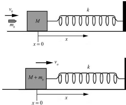
The resulting motion of the block and bullet is simple harmonic motion.
