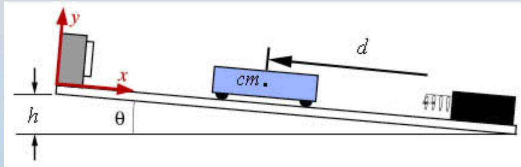
An object of mass  $m$  slides down a plane that is inclined at an angle  $\theta$  from the horizontal. The object starts out at rest. The center of mass of the cart is a distance  $d$  from an unstretched spring with spring constant  $k$  that lies at the bottom of the plane.
