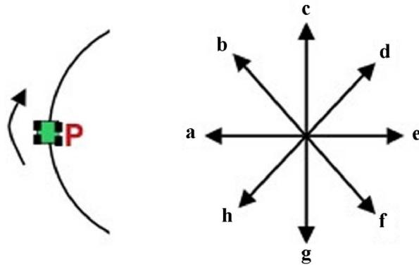
**Answer f.** Since the object is slowing down, the vector describing its acceleration vector has both a tangential and radial component vectors. The radial component vector points inward and the tangential component vector points opposite the direction of its velocity, so the arrow f in the figure best describes the vector sum.
