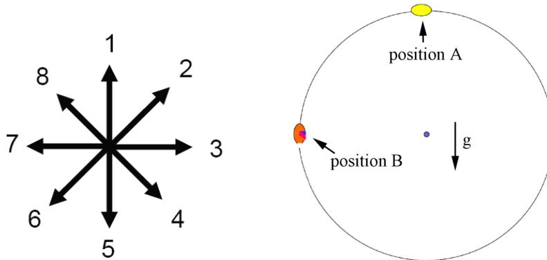
**Solution (4):** The bead is speeding up at position B therefore it has a tangential component of the acceleration (pointing downward) and it is traveling in a circular trajectory so it has a radial component of the acceleration pointing towards the center of the circle. Direction 4 best describes the sum of these two components.
