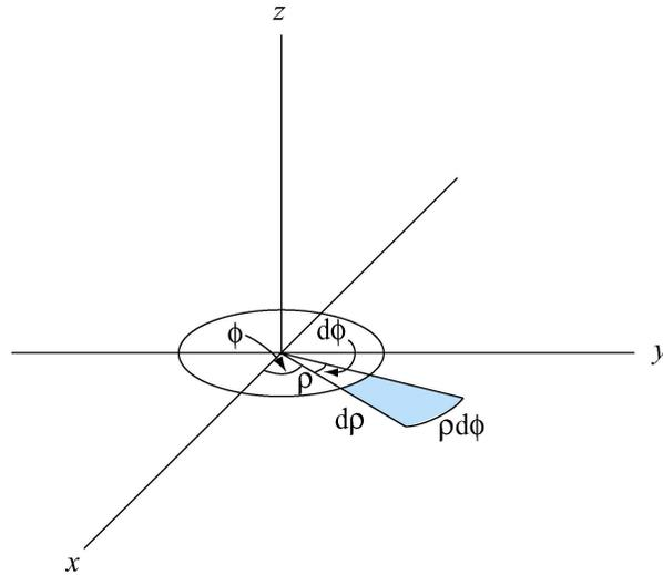
**Figure 9.2.8** Area element for a disc
