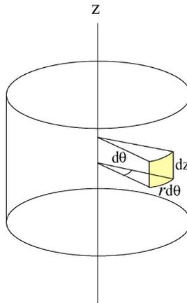
**Figure 9.2.7** Area element for a cylinder
