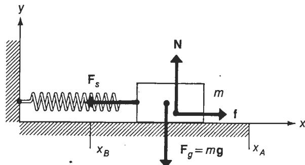
Mass released at  $x = x_A$  with  $v_A = 0$  [Spring is stretched]
