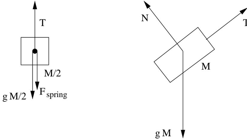
(b) Assume the potential energy is zero when the string is unstretched. After we pull the  $M$  block by a distance  $L$ , the potential energy of the  $M$  block is lower by  $MgL \sin \theta$ , the potential energy of the  $M/2$  block is increased by  $\frac{M}{2}gL$ , and the potential energy of the spring is increased by  $\frac{1}{2}kL^2$ . So the total potential energy of the system is
