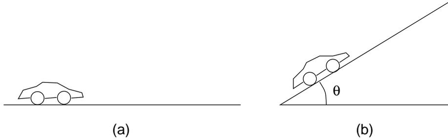
(a) Assume the total resistive force is proportional to the velocity:  $F_{friction} = \alpha v$ . The drag coefficient  $\alpha$  is  $\alpha = 100Ns/m$ . How fast can the car move on a level road? Express the speed in the units of  $m/s$ .
