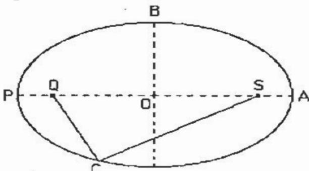
The semi-major axis  $a = OA (= OP)$ , the semi-minor axis  $b = OB$ .  $QO (= OS) = a\epsilon$  ( $\epsilon$  is called the eccentricity). For the special case that the eccentricity is zero, Q, S and O coincide and we have a circle with radius  $R = a = b$ . If two of the three parameters  $a$ ,  $b$ , and  $\epsilon$  are known, the third can be calculated. Convince yourself of this. Keep in mind that  $QC + CS = QB + BS = QA + AS = 2a$ ; that is a property of an ellipse.
