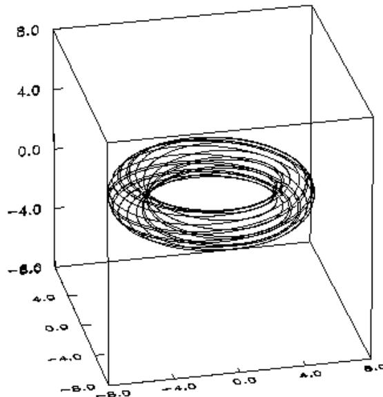
Figure 2.10: Tokamak field lines with rotational transform
