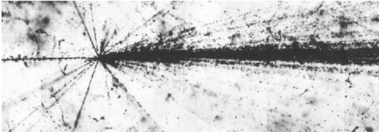
Track structure of a cosmic ray collision in a nuclear emulsion
