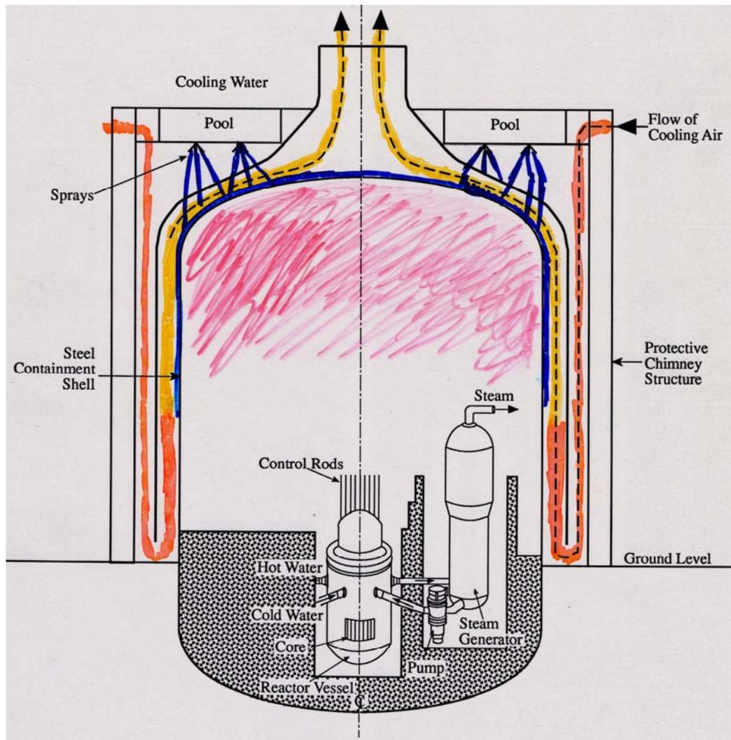
Schematic View of the AP-600 Reactor Concept, showing the containment building and associated cooling systems
