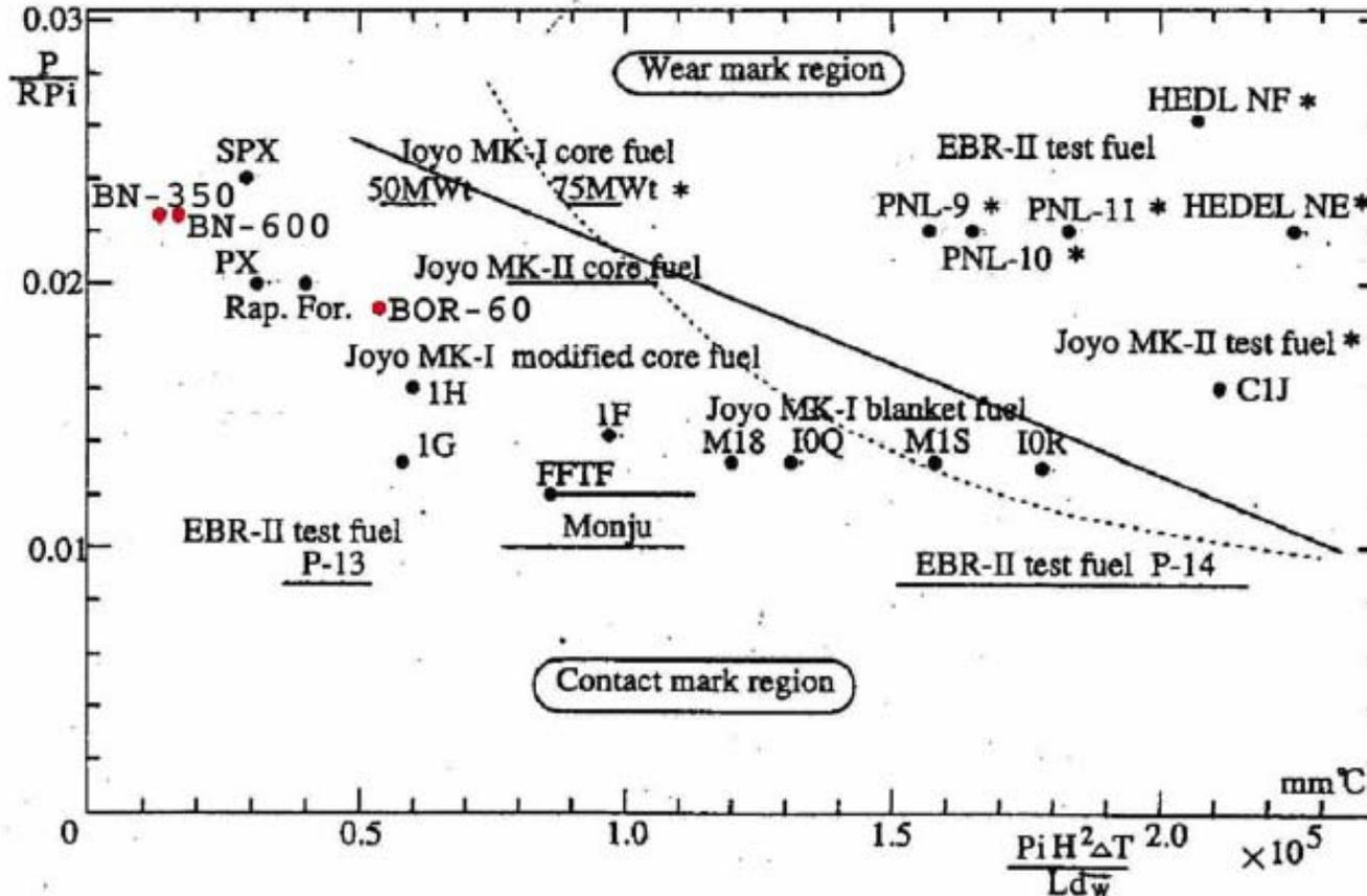
where  $P_i$  is the pitch,  $P$  is the porosity,  $d_w$  is the wire diameter,  $R$  is the number of rings in the bundle,  $\Delta T$  is the temperature drop across the bundle in  $^{\circ}\text{C}$ ,  $H$  is the axial pitch, and  $L$  is the length of the assembly.
