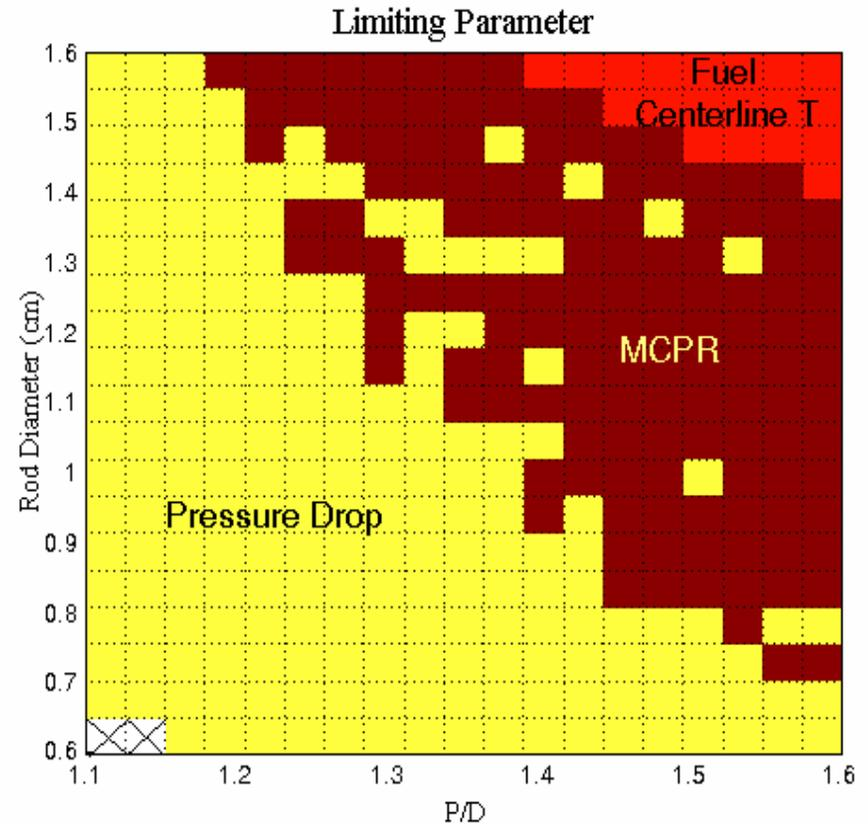
NOTE: 1) vibrations are not limiting, 2)  $\Delta p$  more limiting for Hyd than Ox because of larger number of rods per bundle (Hyd does not contain WRs)
