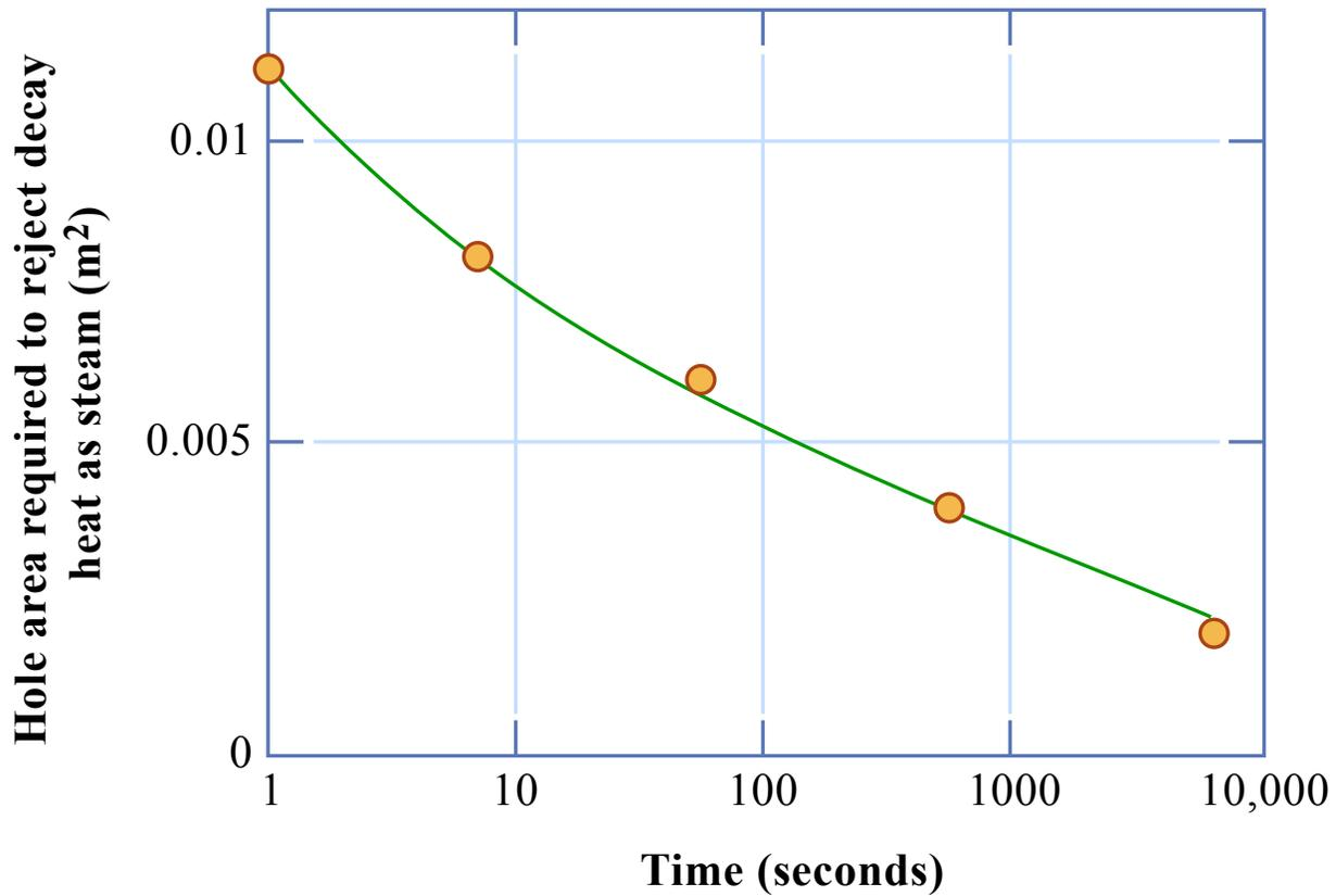
Hole Size to Remove Decay Heat as Steam
