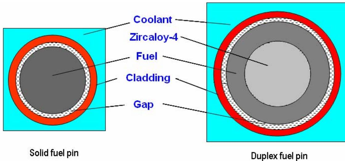
Figure 3: Duplex Fuel Pin Geometry
