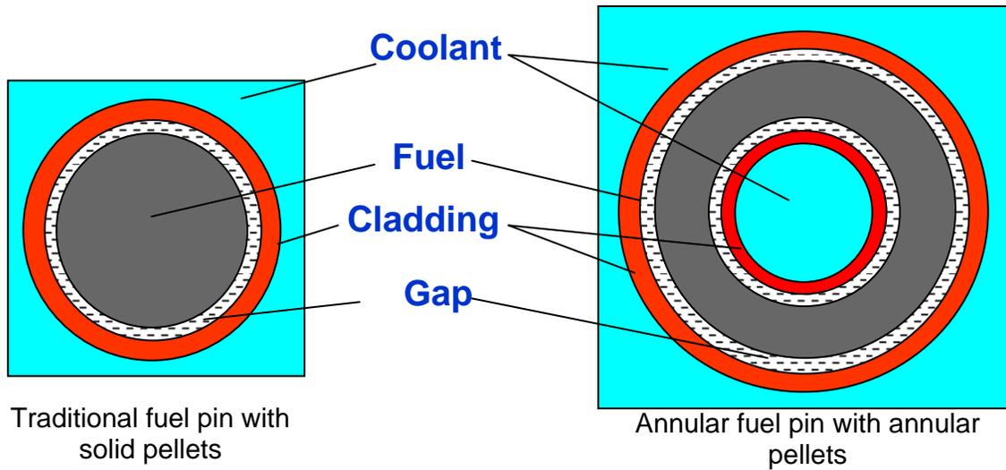
Figure 2: Annular Fuel Pin Geometry (Kazimi)
