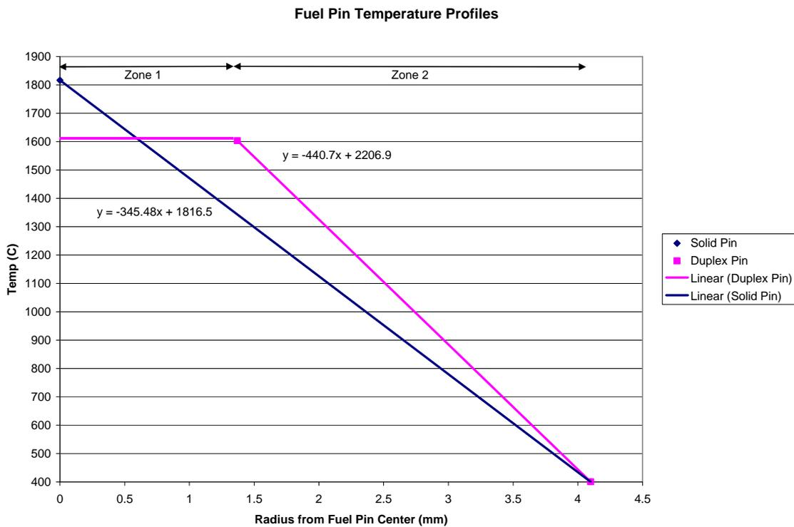
Figure 5: Fuel Pin Temperature Profiles
