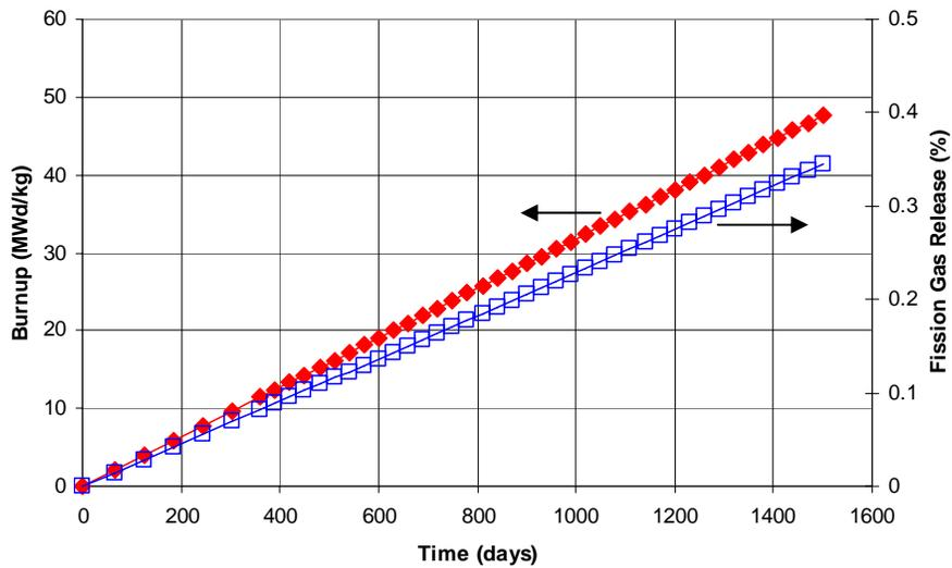
Figure 4. Burnup and fission gas release as a function of time for the FRAPCON case.
