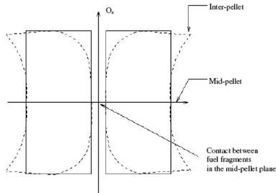
Figure 1. Mechanisms of stress concentration due to pellet radial cracking and hourglassing. [1]
