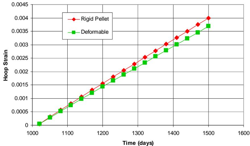
**Figure 8. SiC cladding hoop strain with and without deformable pellet model.**
