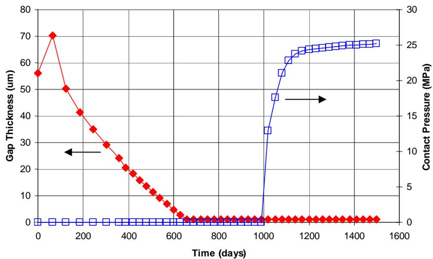
Figure 5. Pellet-cladding radial gap thickness and pellet-cladding contact pressure as a function of time for the FRAPCON case.
