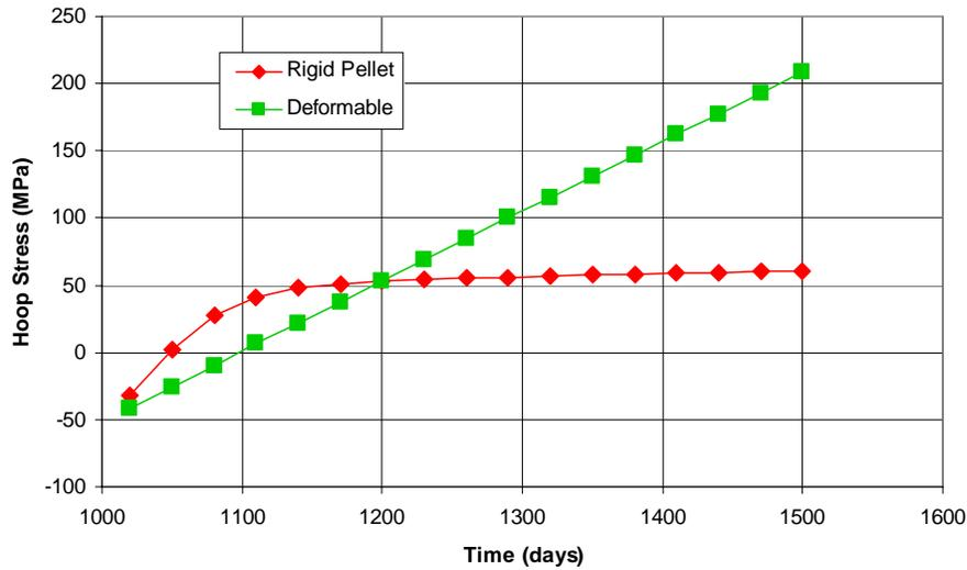
**Figure 7. Zircaloy cladding hoop stress with and without a deformable pellet model.**
