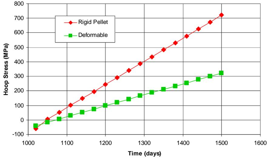
Figure 9. SiC cladding hoop stress and without a deformable pellet model.
