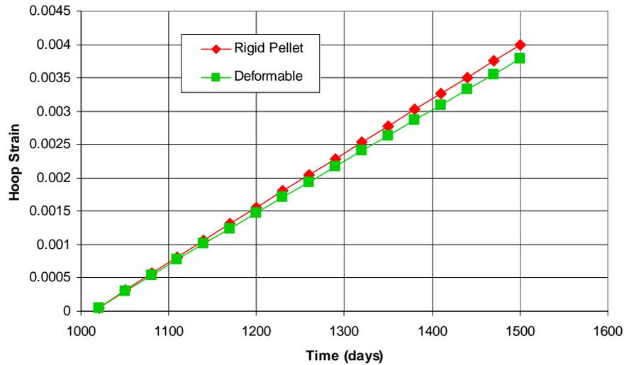
**Figure 6. Zircaloy cladding hoop strain with and without a deformable pellet model.**
