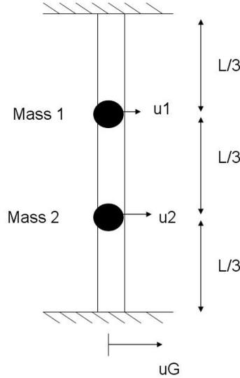
Figure 5: Modeling the pipe: two lumped masses, fixed at  $z=0$  and  $z=L$
