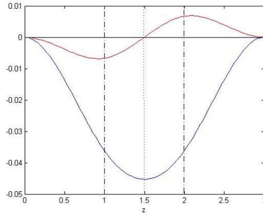
Figure 7: Fundamental modes of the beam: for  $\omega_1$  in blue, for  $\omega_2$  in red.
