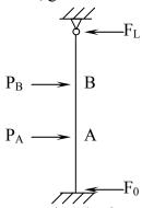
Assuming the forces that act on the supports are  $F_0$  and  $F_L$ , respectively, as in the above figure.
