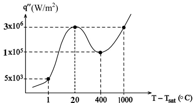
**Figure 4. Boiling curve for a sphere in saturated water at 1 atm.**
