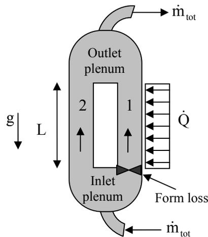
**Figure 3. Parallel channels connected at plena.**
