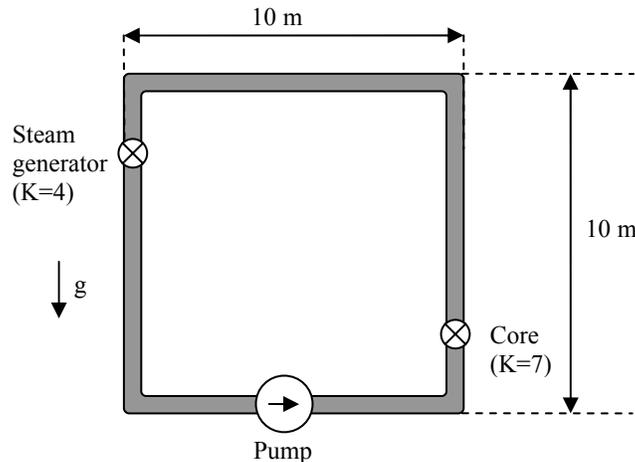
Figure 1. Simplified schematic of the PWR primary system
