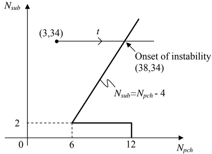
**Figure 4. Trajectory of the channel on the stability map.**
