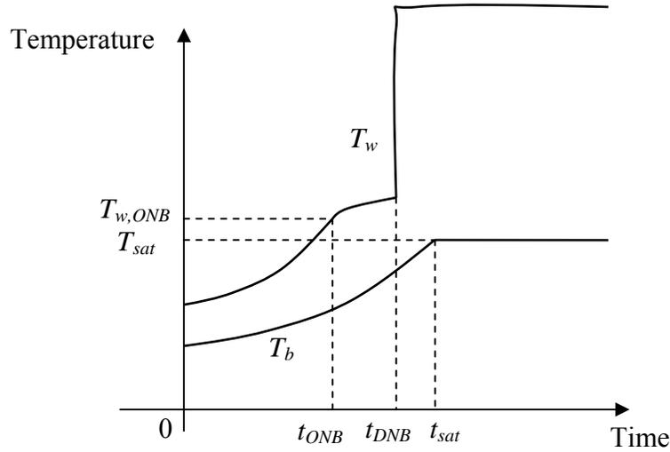
**Figure 3. Time history of the bulk and wall temperatures at the channel outlet (not to scale)**
