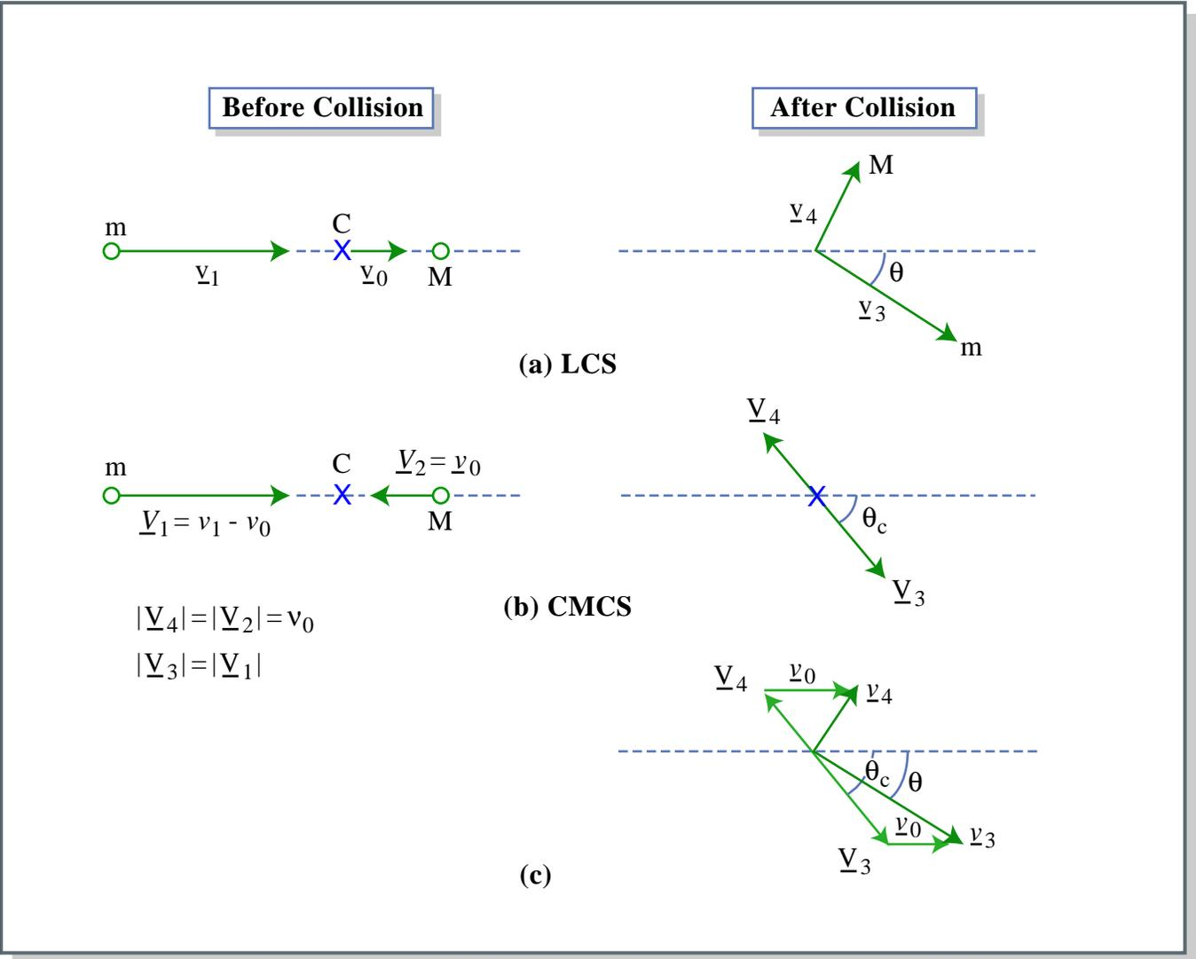
**Fig. 15.2.** Elastic scattering in LCS (a) and CMCS (b), and the geometric relation between LCS and CMCS post-collision velocity vectors (c). Figure by MIT OCW.
