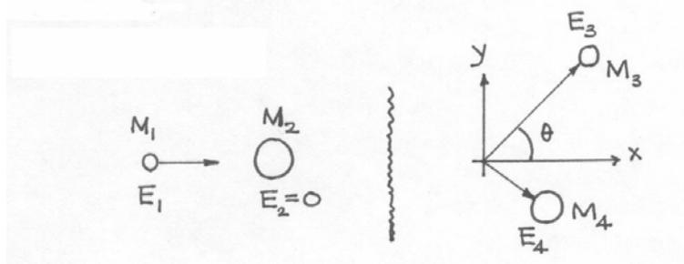
**Fig. 15.1.** A two-body collision between incident particle 1 and target particle 2, which is at rest, leading to the emission of particle 3 at an angle  $\theta$  and a recoiling residual particle 4.
