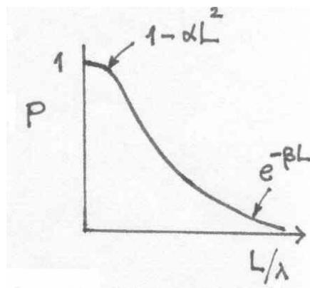
**Fig. 2.** Variation of transmission coefficient (Penetration Factor) with the ratio of barrier width  $L$  to  $\lambda$ , the effective wavelength of the incident particle.
