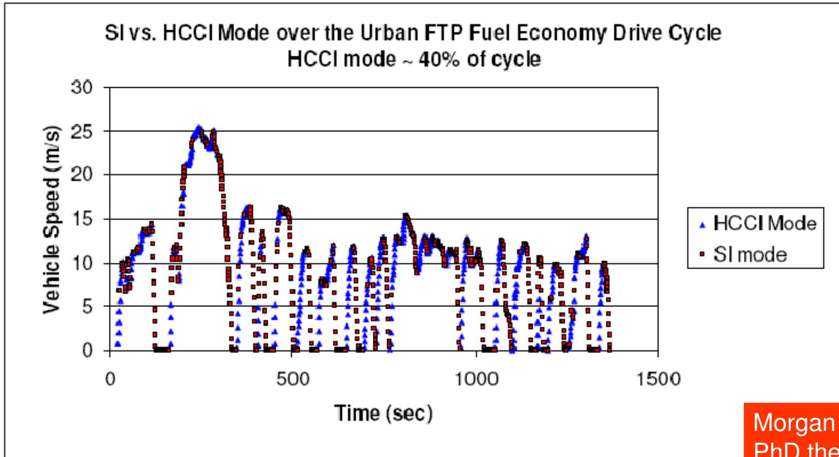
Figure 5.3. Vehicle speed versus time for the FTP Urban Drive Cycle.
