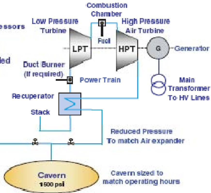
Fig. 1. CAES basic cycle. Source: Alstom Power.
