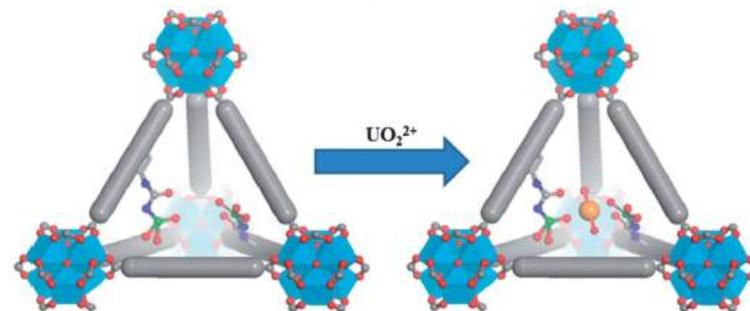
**Fig. 9** Simplified schematic depicting the uranyl-binding pocket formed in the tetrahedron of the MOFs. UO<sub>2</sub><sup>2+</sup> is coordinated in a monodentate fashion to the phosphoryl oxygen. Distances between oxygen range from 4.5–4.8 Å, accommodating U–O bond lengths appropriate for binding motif II–I.
