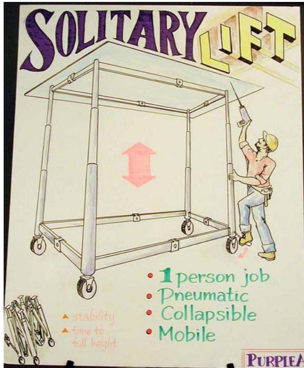
As can be seen, at the time, we were planning on making it pneumatically driven at each of the four pistons in the drawing. However, we quickly realized that this would nearly impossible to actuate and keep perfectly aligned, so we decided to go with a single-piston design:
