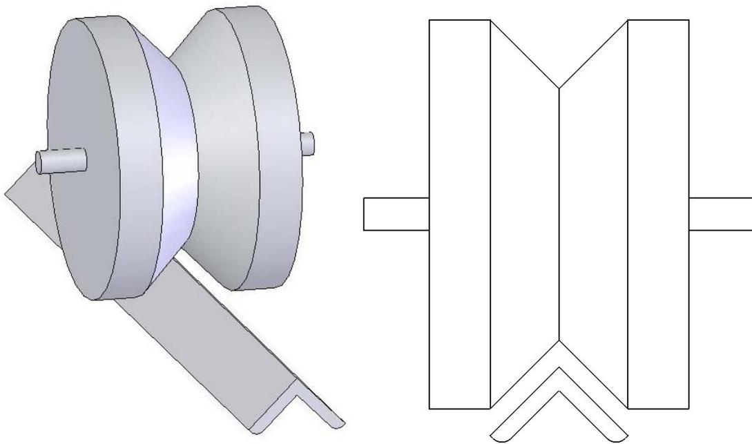
This will provide very accurate positioning, as the neutral position is a stable equilibrium, and the likelihood of undue friction or binding is small. However, it may be more likely to snag feet of actors as they walk over it, and it must also be attached properly to the stage. If the facilities and the material is available, attachment can be as
