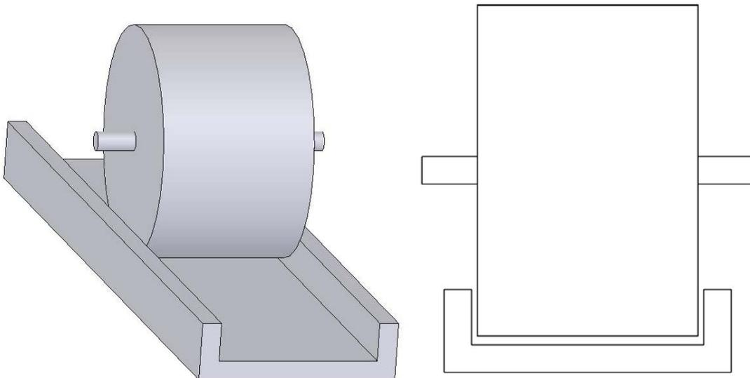
This can be easily achieved, with little more than regular caster, and two strips of wood nailed to the stage on either side of where the caster should travel. Alternatively, if the deck is raised above the stage top, the groove can be recessed into the deck. It could also be accomplished as shown above, with a U-shaped piece. The potential drawbacks of this method are that if the U is too deep, it could bind on the sides of the caster, if sufficient tangential loads were applied to the wagon.
