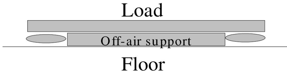
Figure 1: Air caster, section view, air off
