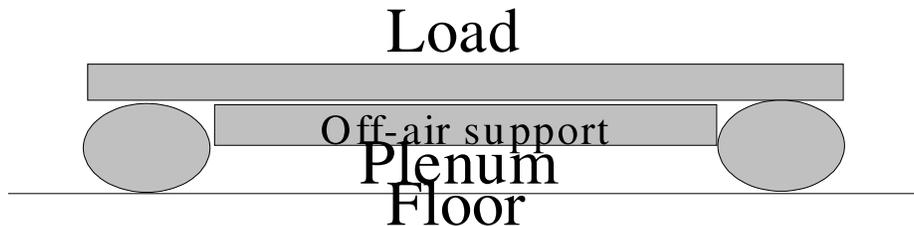
Figure 2: Air caster, section view, air on
