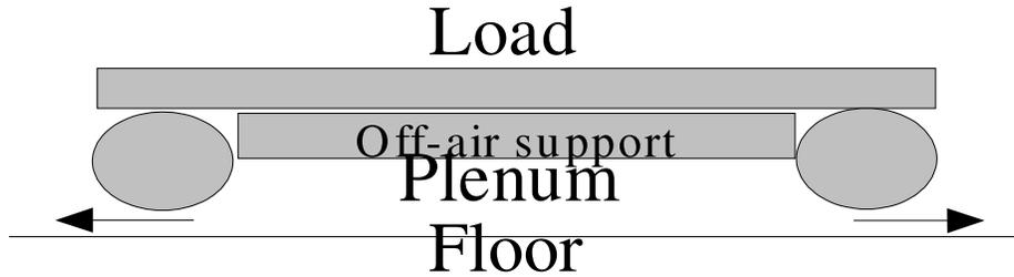
Figure 3: Air caster, section view, floating
