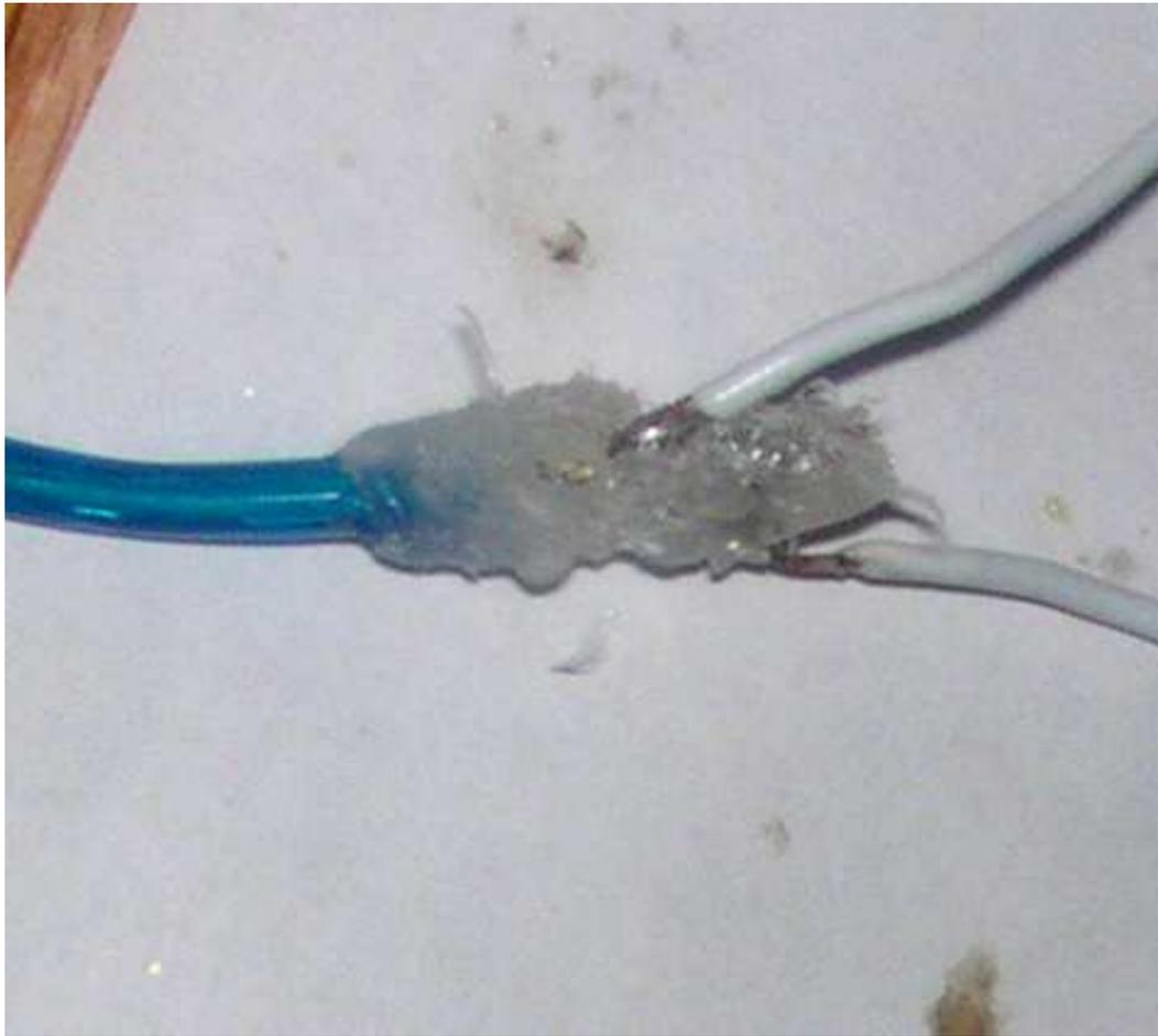
Figure 5: Leads soldered and glued to the inner and outer wires
