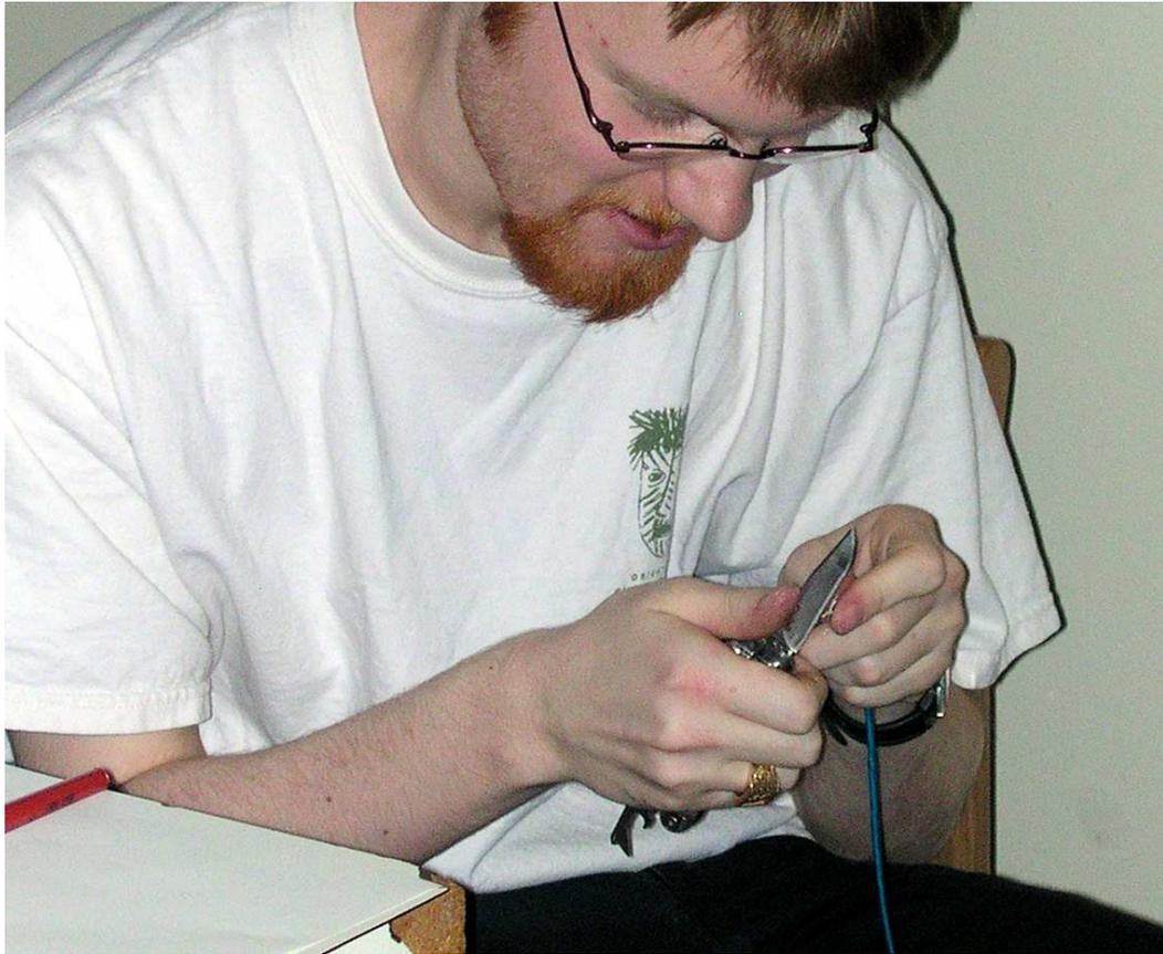
Figure 2: Stripping the outer insulation (and doing unsafe things with knives)
