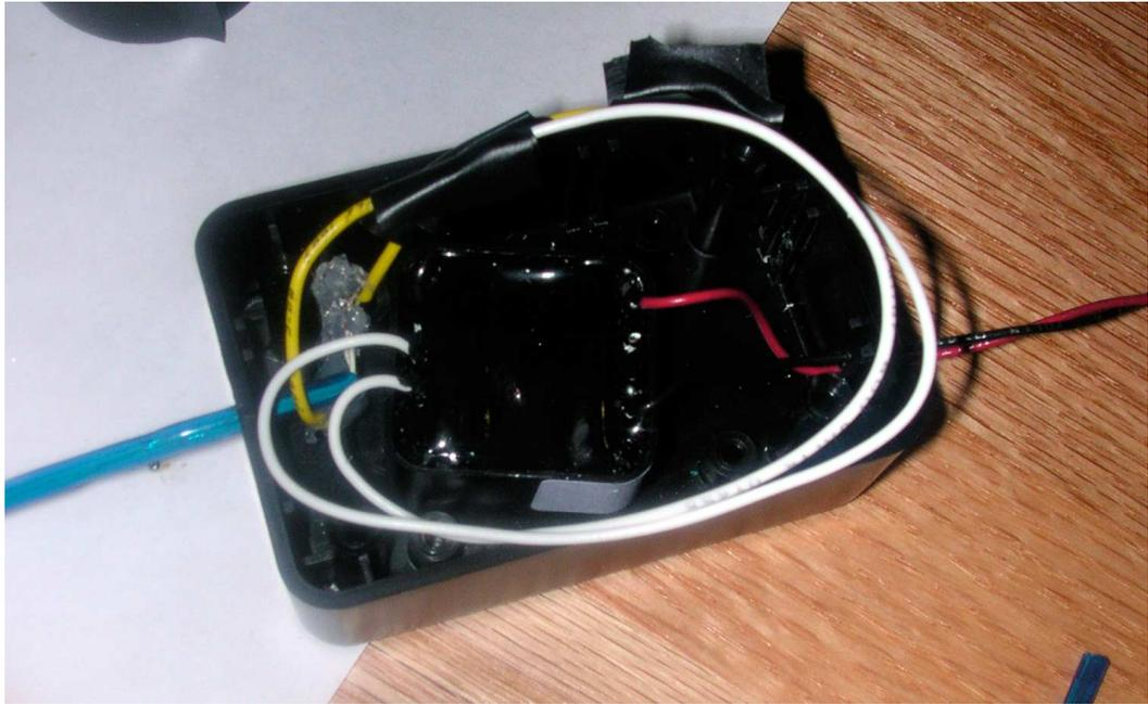
Figure 10: The inverter in place inside the enclosure
