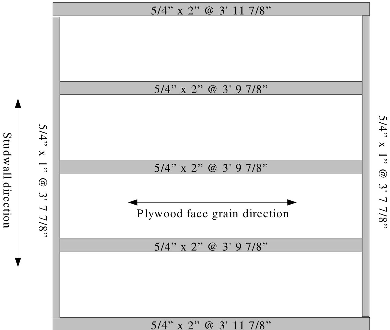
Figure 1: Frame construction layout
