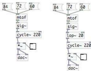
(a) Listen to each of the two sub-patches, one at a time, by using the toggle next to the last [\*~], then vary the message boxes with different pitches. Explain why the patch with the [lop~] sounds different.
