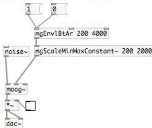
(c) Experiment with this filtered noise patch, triggering the opening and closing of the envelope with the 1 and 0 message boxes. Create a new version that rises to 6000 Hertz in 6 seconds, and falls to 100 Hertz in 3 seconds.
