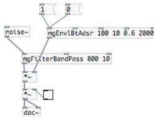
(e) Experiment with this bandpass filtered noise patch. Expand this patch such that there are two noise bands (at 800 and 2000 Hertz) mixed together and that the ADSR has a very slow attack (> 4 sec) and has a very fast release (< 1 sec).
