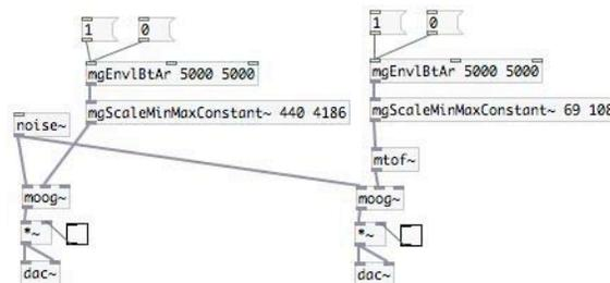
(d) Compare the sonic changes of these two envelope-driven filters, one at a time, while triggering the envelopes. What is the difference in way the filter cutoff frequency moves? Which do you prefer?
