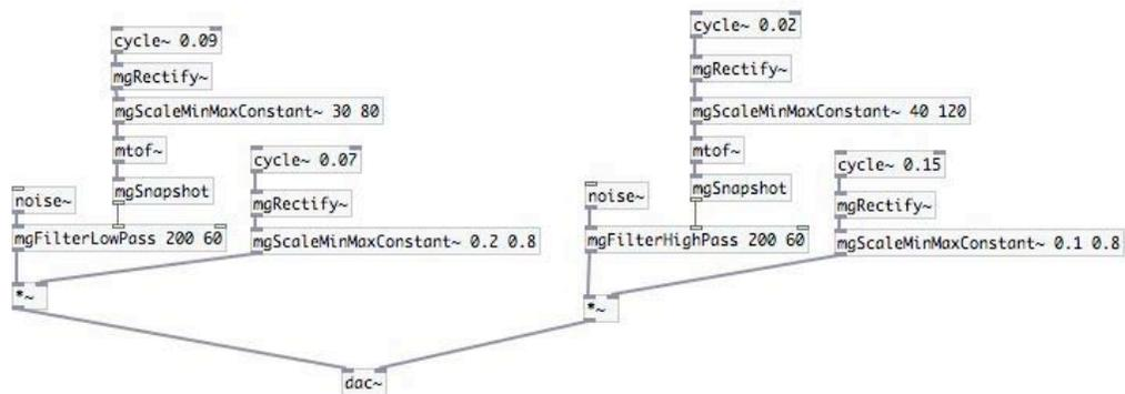
(a) This patch creates waves of noise, where both the timbre of the noise and the amplitude of the noise are smoothly varied with [cycle-] objects. Recreate this patch and elaborate it by adding more noise bands, using different filters, and/or controlling filter and amplitude parameters in different ways.
