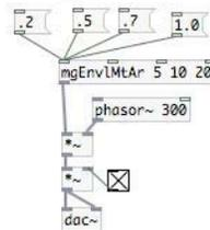
(f) Listen to the enveloped phasor with different peak amplitudes, as triggered with the message boxes. Provide new values to these message boxes that will provide what sound like evenly-spaced gradations of amplitude.
