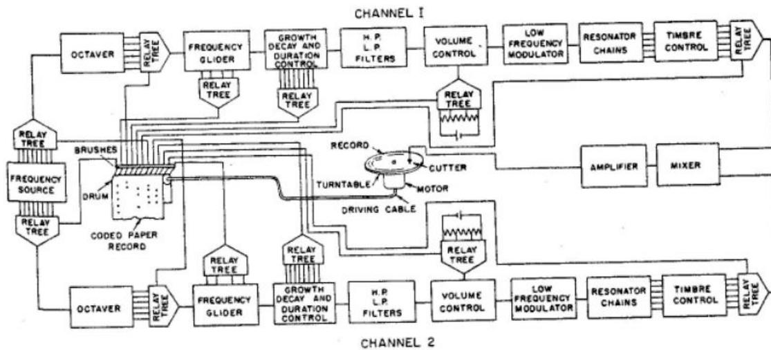
FIG. 2. Schematic diagram of the electronic music synthesizer.
