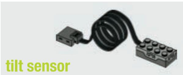
The tilt sensor can be used to determine orientation, where 0 is flat, 1 is down, 2 is right, 3 is up, and 4 is left.
