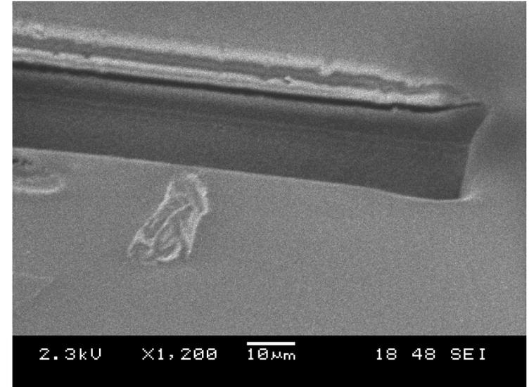
'Ploughing' in plastic caused by differential thermal contraction of Si mold and polymer substrate (embossing at  $\sim 130$  °C)
