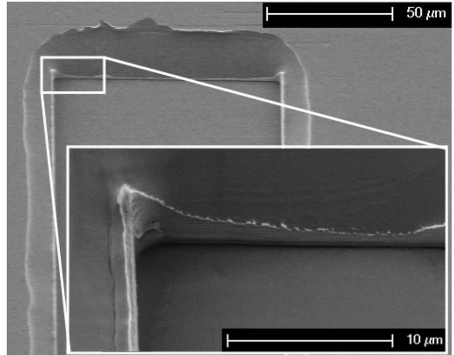
SEM of end of 100  $\mu\text{m}$  wide x 15  $\mu\text{m}$  deep channel, de-molded at 120  $^{\circ}\text{C}$  after 10 minutes
