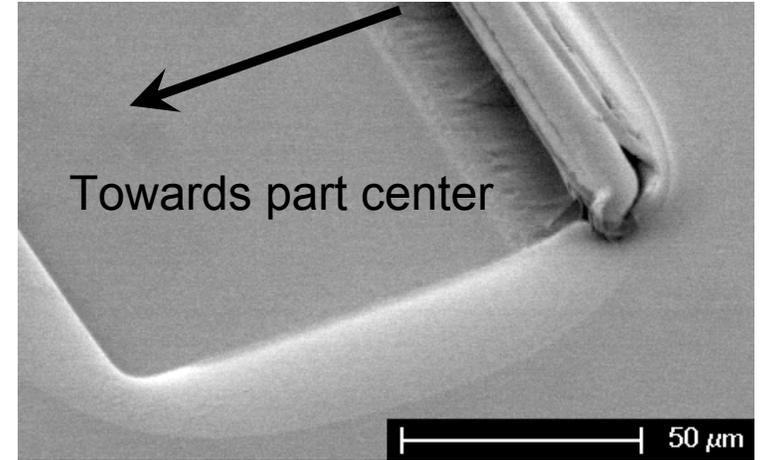
SEM of end of 100  $\mu\text{m}$  wide by 15  $\mu\text{m}$ -deep trench, de-molded at 50 °C
