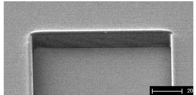
SEM of end of 100  $\mu\text{m}$  wide by 15  $\mu\text{m}$ -deep trench, de-molded at 110 °C
