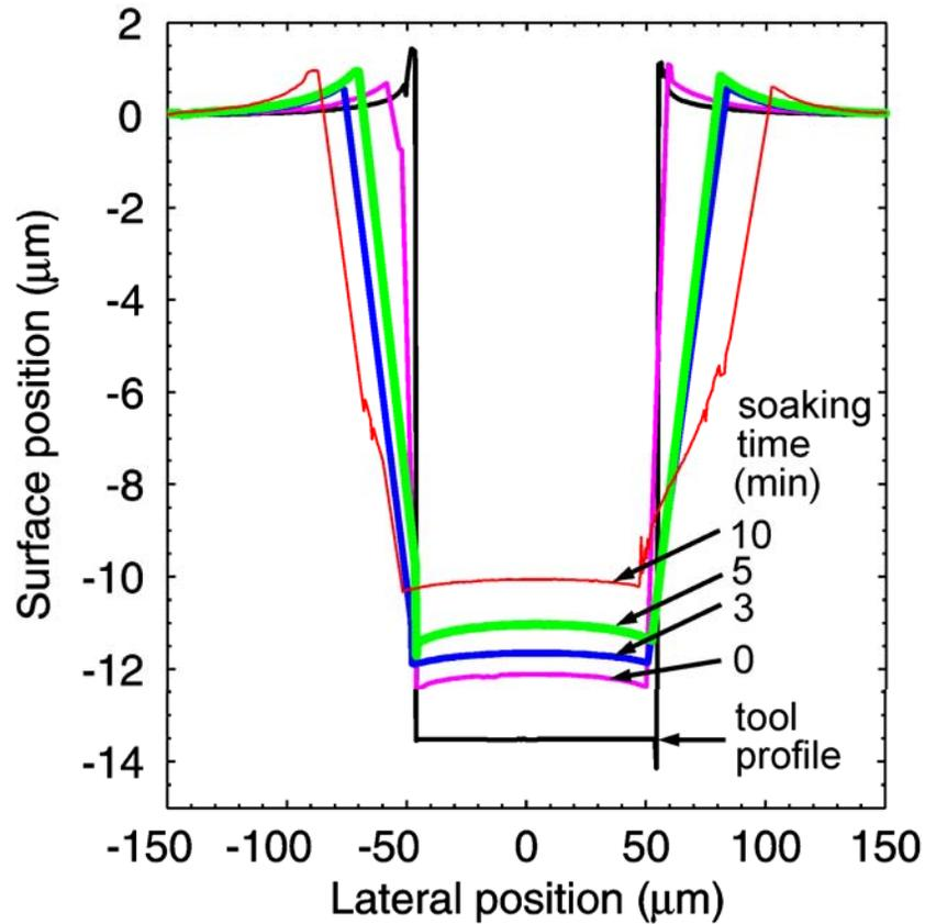
Cross-sections of 100  $\mu\text{m}$  wide by 15  $\mu\text{m}$ -deep square. Obtained by scanning white-light interferometry.
