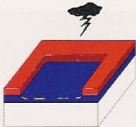
**5.** A layer of silicon dioxide is etched away by a gas plasma, leaving only a thin insulating layer.
