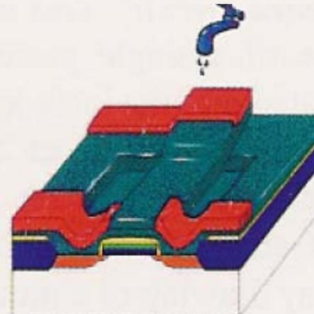
**23.** A chemical solvent removes the exposed photoresist, creating a photoresist pattern above the aluminum.
