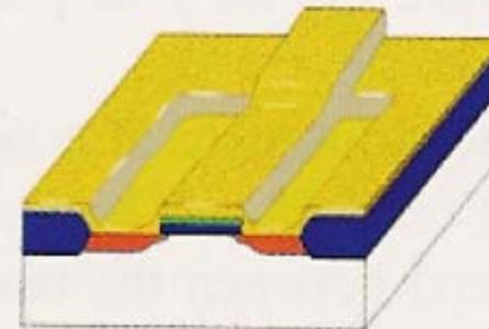
**15.** A layer of photoresist is deposited on the wafer, in preparation for metal contacts to the source, drain, and gate of the transistor.
