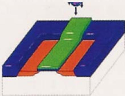
**13.** Phosphorous atoms are implanted in the positively doped silicon substrate, forming the source and drain as negatively charged wells (orange).
