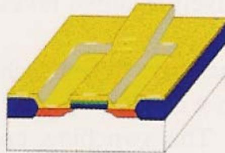
**14.** A new layer of silicon dioxide is deposited. It will insulate the transistor structure, except for metal contacts that will be added.
