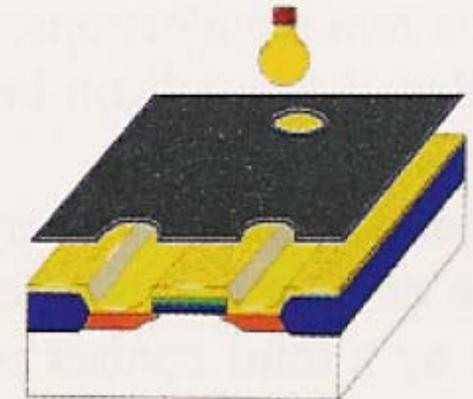
**16.** Light shining through a patterned mask chemically alters most of the photoresist, except three small areas for metal contacts.
