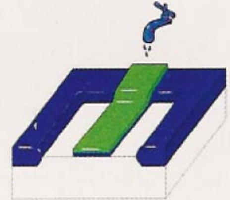
**12.** A chemical solvent washes away the remaining photoresist, leaving the polysilicon transistor gate structure (green).
