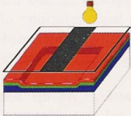
**9.** Light shining through a new patterned mask chemically changes the photoresist that is exposed to the light.
