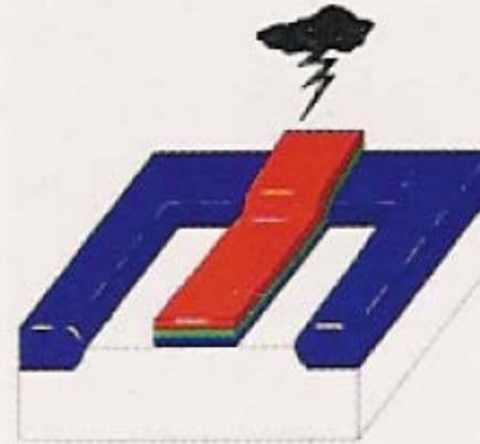
**11.** Polysilicon and a thin layer of silicon dioxide are removed by etching, exposing the underlying silicon substrate (white).
