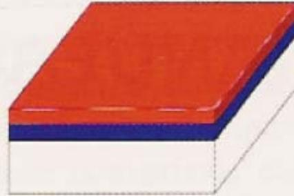
**2.** A layer of photoresist (red), sensitive only to ultraviolet light, is deposited on the wafer.
