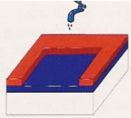
**4.** A chemical solvent washes away the exposed photoresist, leaving a patterned layer of photoresist above the silicon dioxide.
