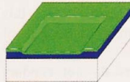
**7.** A layer of polysilicon (green) is deposited on the wafer. It will form the transistor gate for transmitting electrical current.
