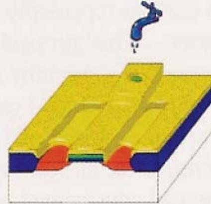
**19.** A chemical solvent removes the photoresist. The negatively doped source and drain (orange) and the polysilicon gate (green) are opened to metal contacts.
