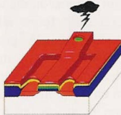
**18.** Dry etch removes the exposed silicon dioxide, opening shafts to the negatively doped substrate and the polysilicon.
