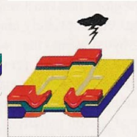
**24.** The exposed aluminum is etched away, leaving aluminum "wires" that will carry current to and from the transistor.
