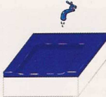
**6.** A chemical solvent washes away the remaining photoresist, leaving an uneven silicon dioxide surface.
