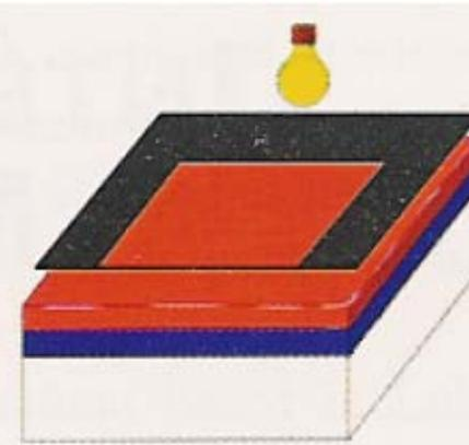
**3.** Light shining through a mask of chromium (black)-patterned glass chemically changes the exposed photoresist.
