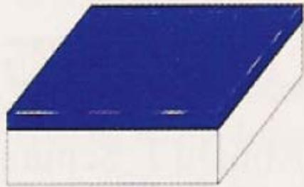
**1.** The transistor's insulating layer of silicon dioxide (blue) is grown in a hot furnace on a positively doped silicon substrate on a wafer.
