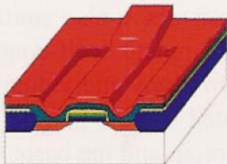
**21.** A fourth layer of photoresist is deposited on the wafer.
