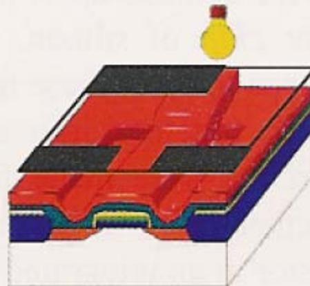
**22.** Light shining through the fourth patterned mask chemically changes the exposed photoresist.
