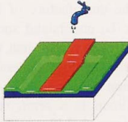
**10.** A chemical solvent removes the exposed photoresist, leaving a patterned layer of photoresist above the polysilicon.
