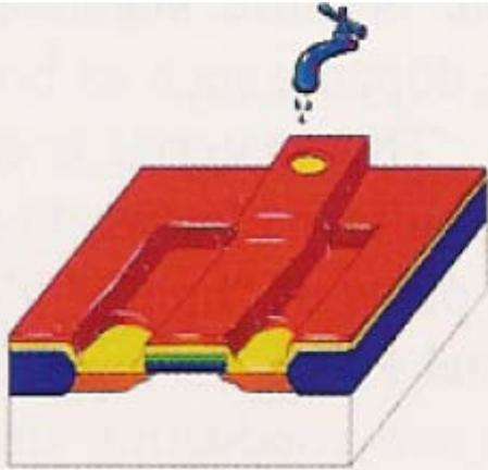
**17.** A chemical solvent removes the exposed photoresist, opening access to three small areas of silicon dioxide.
