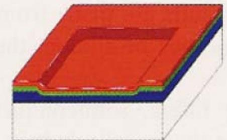
**8.** A new layer of photoresist is deposited on the polysilicon layer.
