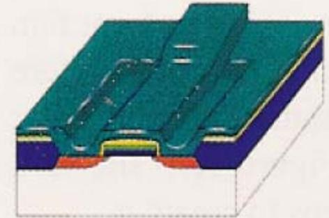
**20.** Aluminum (blue-green) is deposited over the surface and inside the three shafts. It will provide electrical connections.
