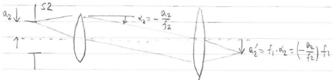
$$\text{FOV} = \underbrace{\left| \frac{a_2'}{f_1} \right|}_{\text{limiting angle of the chief ray}} = \frac{a_2 f_1}{f_2 f_1} = \frac{a_2}{f_2} \quad (\text{half-field})$$
