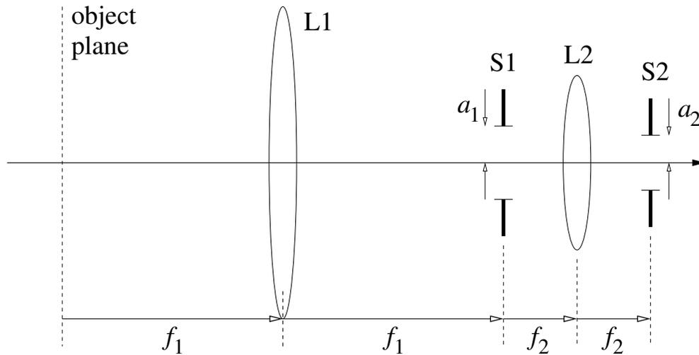
**2. Aperture and field stops in a telescope with finite conjugates** For the telescope configuration shown above, where lenses L1 and L2 have focal lengths  $f_1$ ,  $f_2$ , respectively, the object plane and two stops S1 and S2 of half-sizes  $a_1$ ,  $a_2$ , respectively, are at the locations shown,
