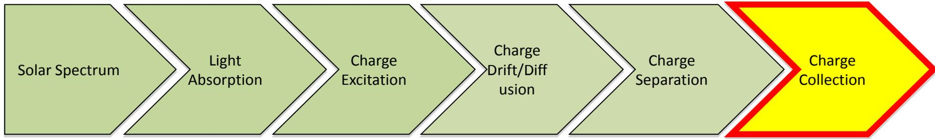
$$\eta_{\text{total}} = \eta_{\text{absorption}} \times \eta_{\text{excitation}} \times \eta_{\text{drift/diffusion}} \times \eta_{\text{separation}} \times \eta_{\text{collection}}$$
