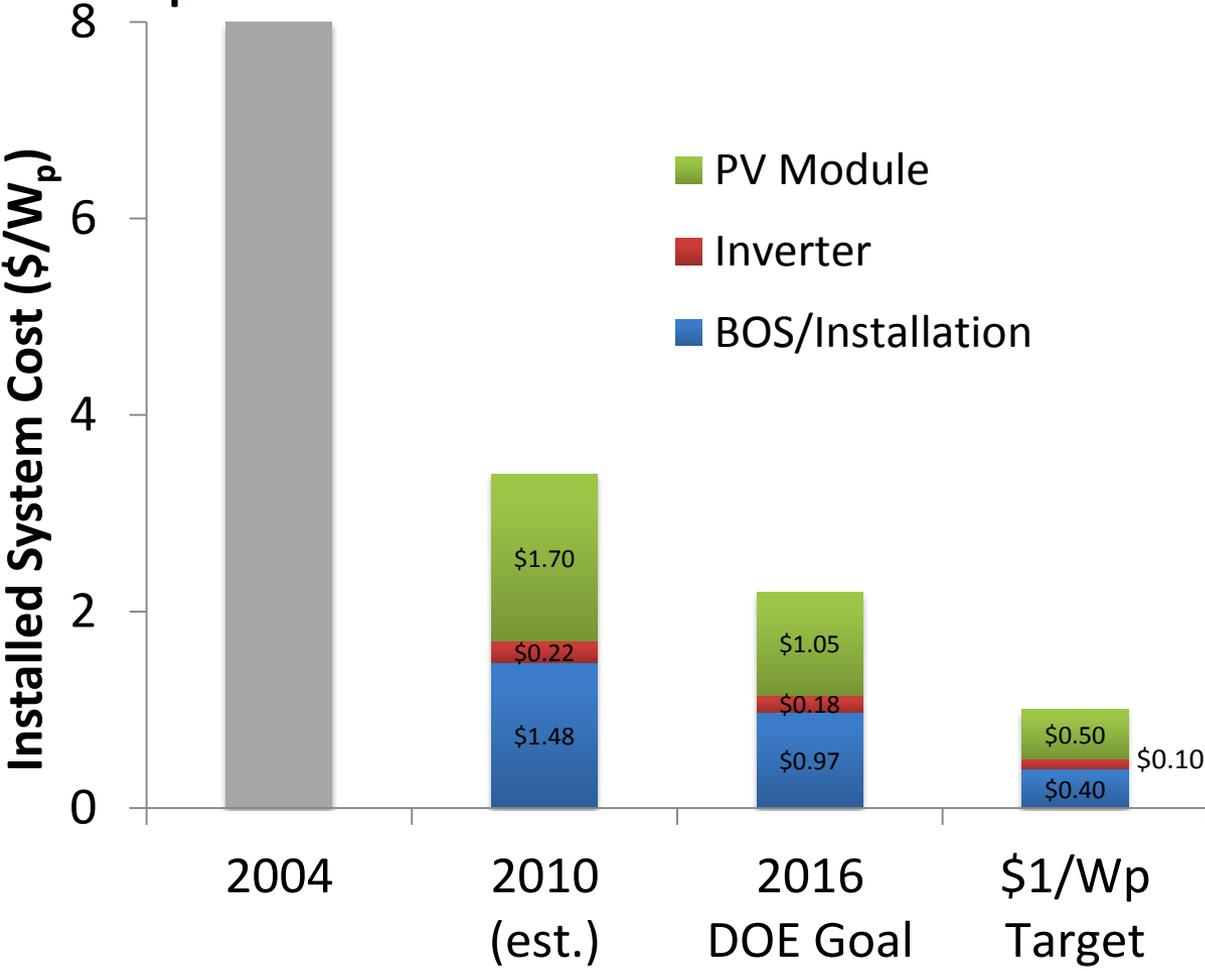
>3x PV module cost reduction necessary for \$1/W<sub>p</sub>.
