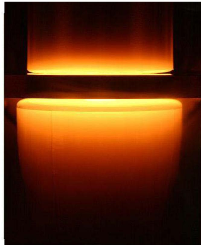
*Diameters and rotation speeds of the polysilicon ingot and the growing single crystals can be different*
