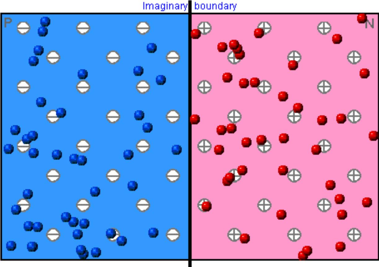
With the P and N type materials separated the carriers diffuse around randomly.
