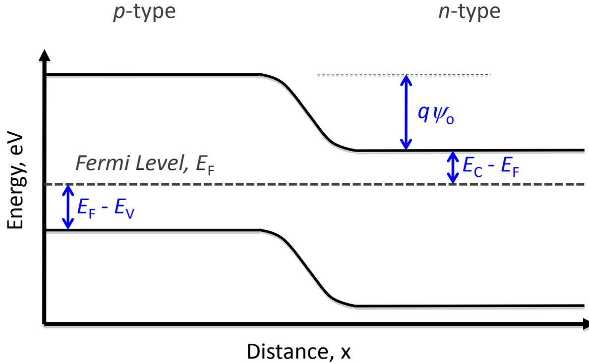
$$\begin{aligned} q\psi_0 &= E_g - (E_F - E_V) - (E_C - E_F) \\ &= \frac{kT}{q} \ln\left(\frac{N_A N_D}{n_i^2}\right) \end{aligned}$$
