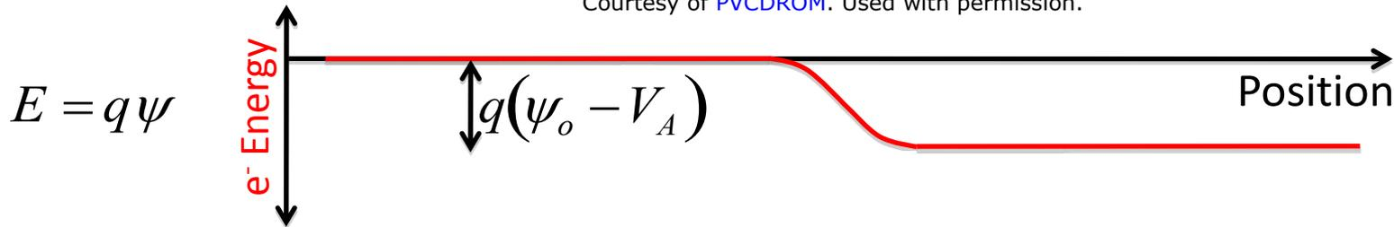
1. When light creates an electron-hole pair, a *pn*-junction can separate the positive and negative charges because of the built-in electric field.
