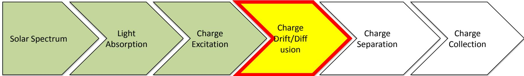
$$\eta_{\text{total}} = \eta_{\text{absorption}} \times \eta_{\text{excitation}} \times \eta_{\text{drift/diffusion}} \times \eta_{\text{separation}} \times \eta_{\text{collection}}$$
