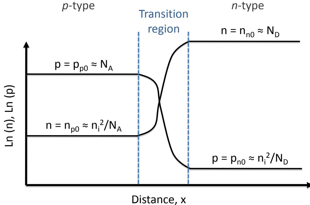
Approximation 1: Device can be split into two types of region: quasi-neutral regions (space-charge density is assumed zero) and the depletion region (where carrier concentrations are small, and ionized dopants contribute to fixed charge).
