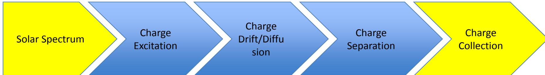
$$\eta_{\text{total}} = \eta_{\text{excitation}} \times \eta_{\text{drift/diffusion}} \times \eta_{\text{separation}} \times \eta_{\text{collection}}$$
