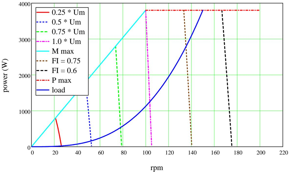
So ... as observed in the text: "The operational envelopes show that a DC motor is very suited to drive a propeller for ship propulsion."
