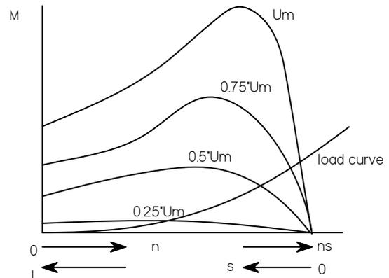
fig. 9.21 Torque - speed curve induction motor varying supply voltage, from Woud
