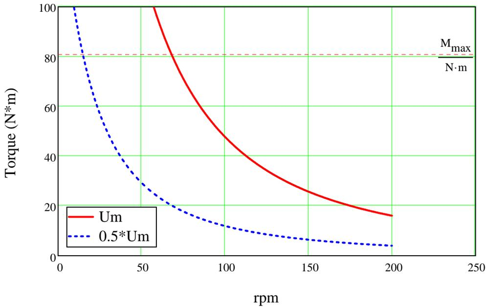
motor suitable for traction purposes - high torque at low rpm
