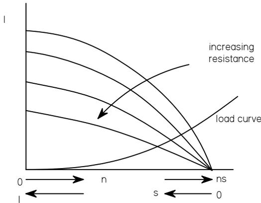
fig. 9.20B Current - speed curve varying rotor resistance from Woud
