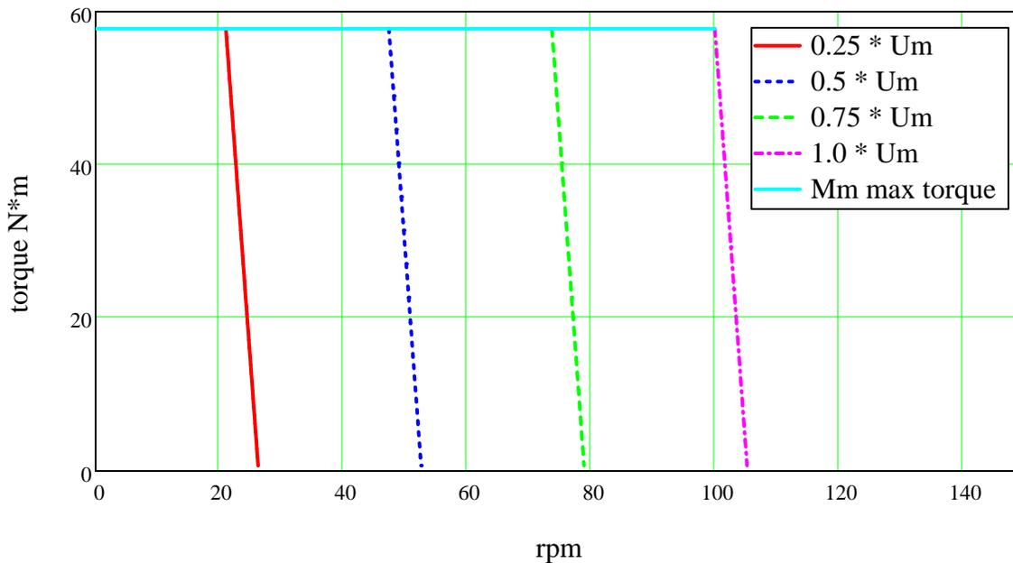
additional operating envelope is available beyond design rpm by reducing the field strength  $\Phi$ . But the region is limited by the maximum power available
