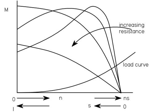
fig. 9.20A Torque - speed curve varying rotor resistance from Woud
