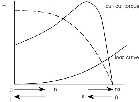
fig. 9.18 Torque - speed curve induction motor from Woud
