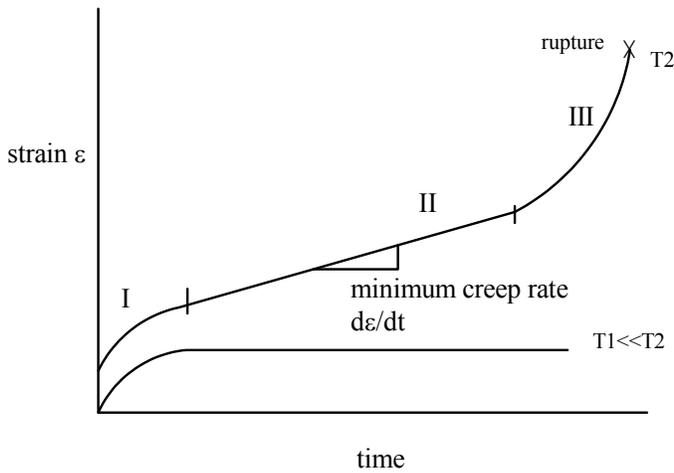
stage I: primary creep: rapid initial deformation
