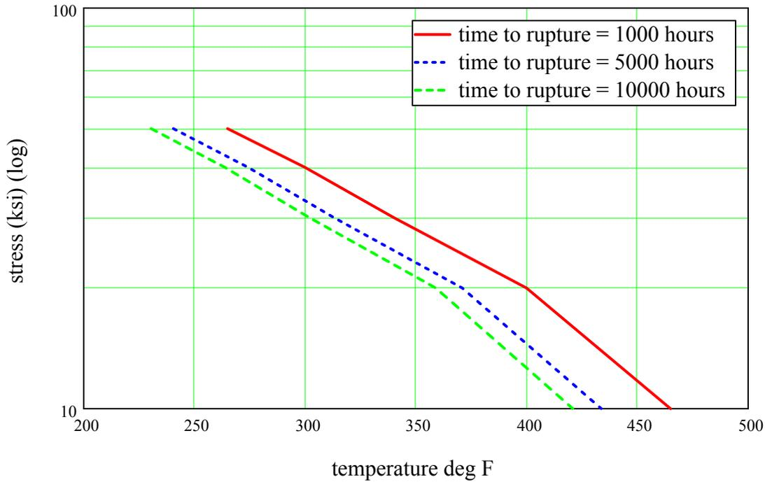
These curves are difficult to use so researchers proposed a parameter that collapses data empirically. E.g. these data can be represented on a Master Curve for Creep using the Larson-Miller (or another similar parameter). The plots lack smoothness due to manual extraction of data.
