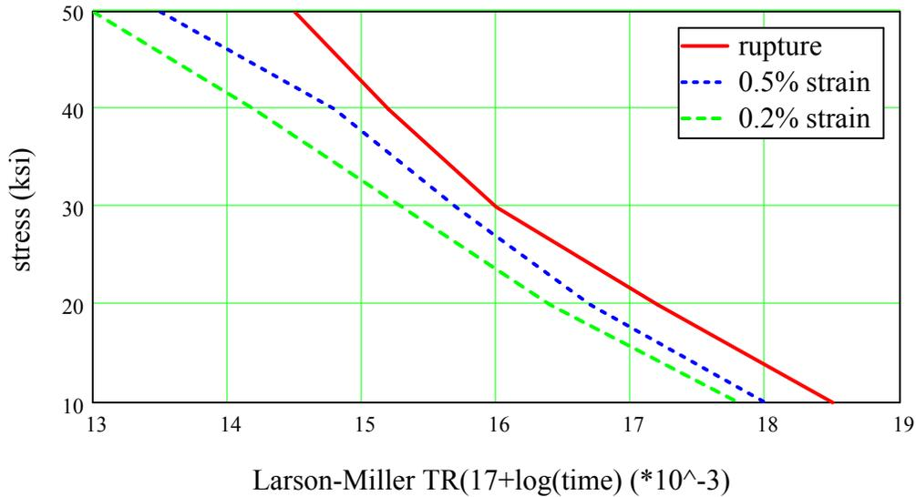
The Larson Miller parameter combines temperature and times (rupture, strain) as follows:
