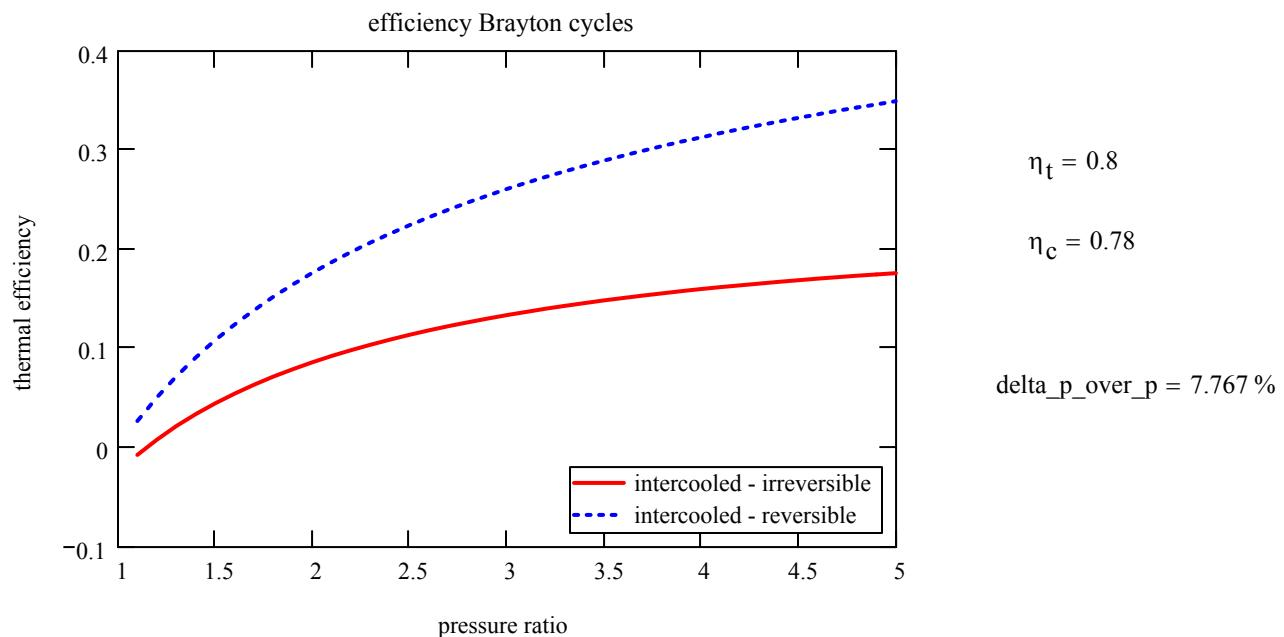
$$\text{ratio}_{rev} = \frac{\text{work}_{comp}}{\text{work}_{turb}} = \frac{(N+1) \cdot (T_{2S} - T_1)}{T_3 - T_4}$$
