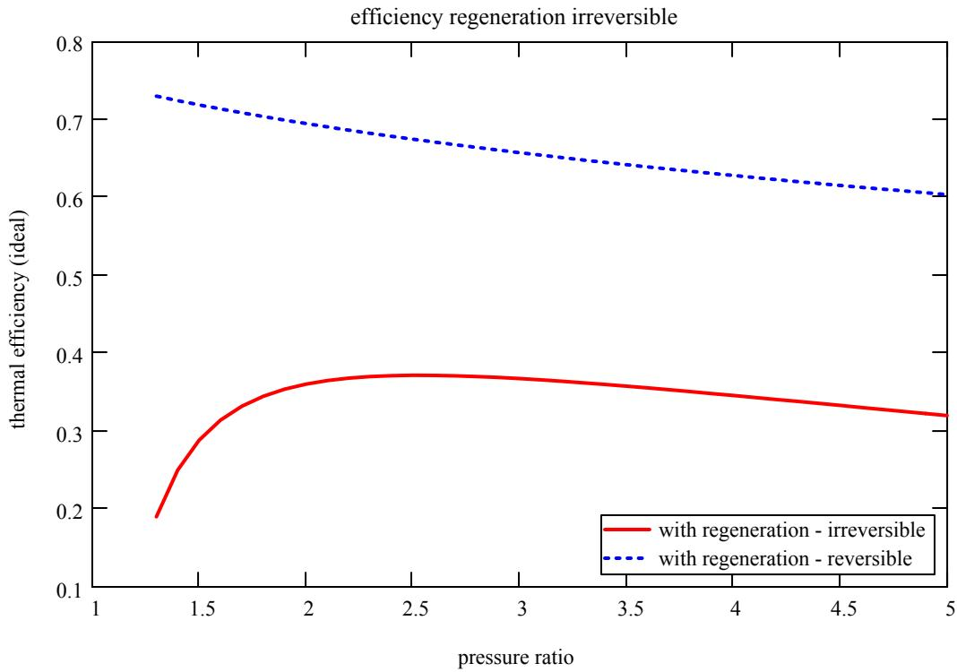
also look at magnitude of compressor work compared to turbine, say for  $pr = 2$  (since these states are the same for w & w/o regeneration, the work is also the same)
