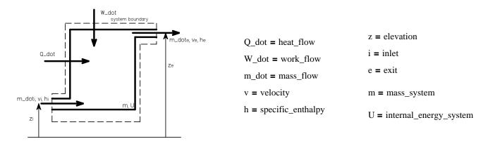
First law: change of energy within the system equals the heat flow into the system, minus the work flow delivered by the system, plus the difference in the enthalpy, H, kinetic energy  $E_{kin}$  and potential energy  $E_{pot}$  of the entering and exiting mass flows.
