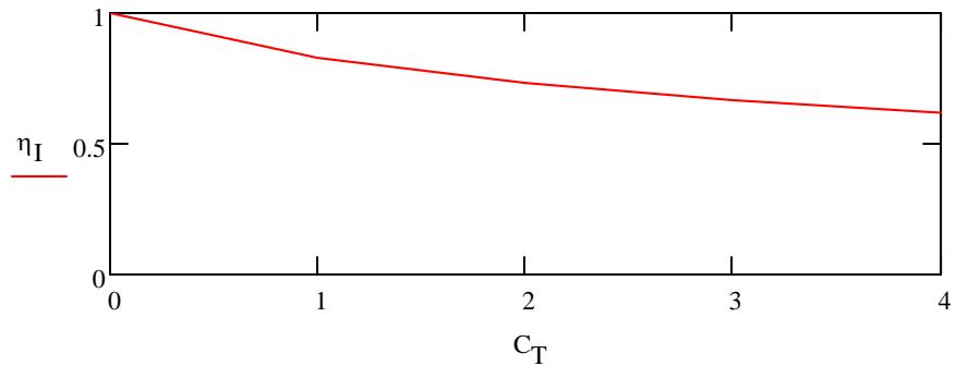
Observations: 1). Propeller at high load coefficient  $C_T$  less efficient
